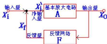
$$\text{由于: } X'_i = X_i - X_f \quad \text{所以: } X_o = A(X_i - X_f) = A(X_i - FX_o) = AX_i - AFX_o$$
