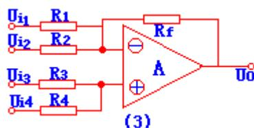
$$U_o = R_f \left( \frac{U_{i3}}{R_3} + \frac{U_{i4}}{R_4} - \frac{U_{i1}}{R_1} - \frac{U_{i2}}{R_2} \right)$$
