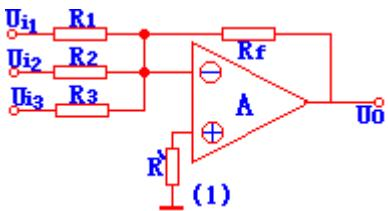
$$U_o = -\left(\frac{R_f}{R_1}U_{i1} + \frac{R_f}{R_2}U_{i2} + \frac{R_f}{R_3}U_{i3}\right)$$
