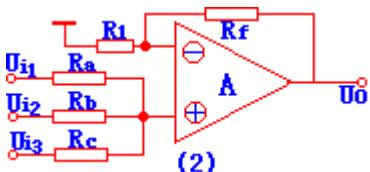
$$U_o = R_f \left( \frac{U_{i1}}{R_a} + \frac{U_{i2}}{R_b} + \frac{U_{i3}}{R_c} \right)$$
