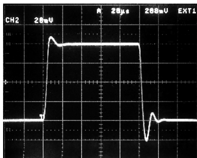
Figure 22. Small Signal Pulse Response, G = +5 , R_L = 20 k\Omega , C_L = 50 pF
