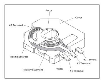
Heat both the terminal and the land at the same time so that the wire solder melts quickly. This will reduce deformation of the resin substrate of the product due to heat transmitted from the terminals.
