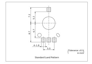
This product has two #2 terminals, at positions A and B to ensure flexibility of mounting on the board to cope with various wiring layouts.
