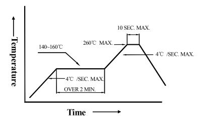
3). DIP soldering (Wave Soldering):
