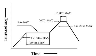
3). DIP soldering (Wave Soldering):
