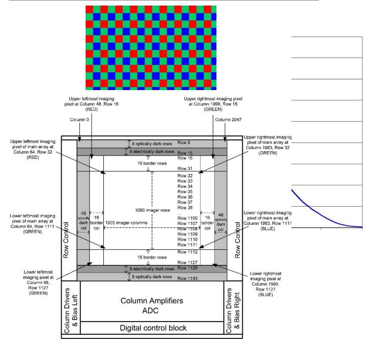
The Bayer pattern RGB Color Filter Array (CFA) covers the 1952 (H) x 1112 (V) imaging pixels and extends 2 pixels deep into the dark pixels region on all 4 sides. Even numbered rows are Red/Green, with even columns Red and odd columns Green. Odd numbered rows are Green/Blue, with even columns Green and odd columns Blue
