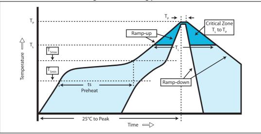
Figure 11. Soldering profiles
