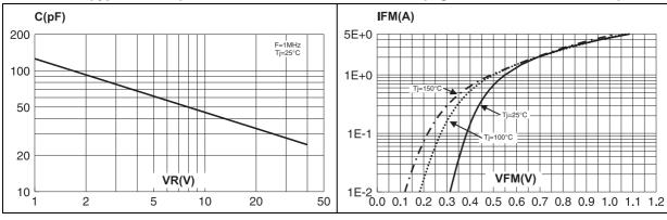
Figure 9. Forward voltage drop versus forward current (low level, maximum values)
