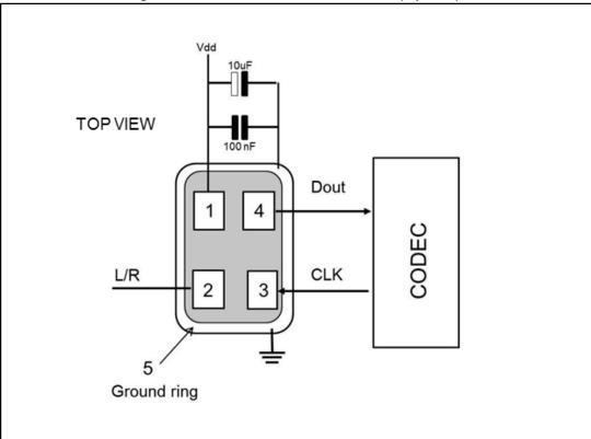
Figure 4: MP34DT04 electrical connections (top view)
