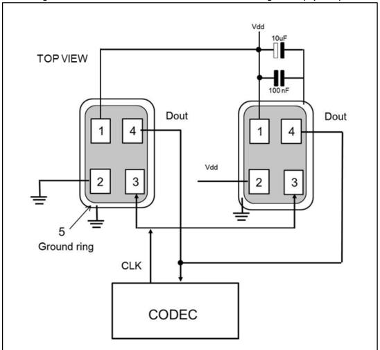
Figure 5: MP34DT04 electrical connections for stereo configuration (top view)
