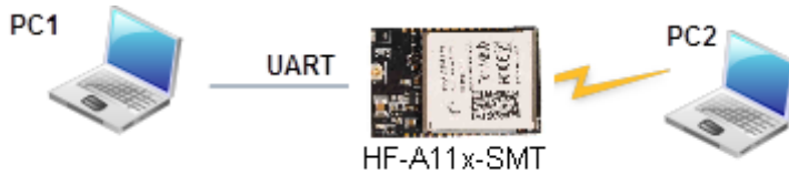
Figure 29. AP Interface Debug Connection
