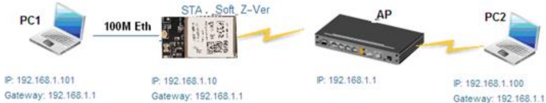
Figure 20. HF-A21-SMT Ethernet Interface Networking (As STA, Z-Ver)
