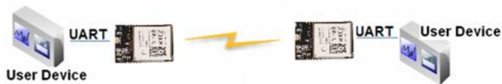
Figure 21. HF-A21-SMT Transparent Transmission Demo
