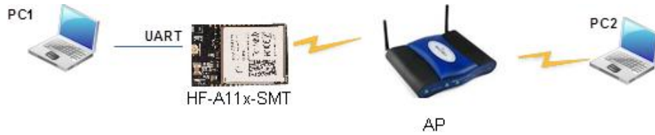
Figure 28. STA Interface Debug Connection
