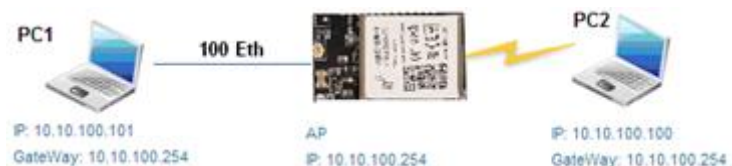
Figure 18. HF-A21-SMT Ethernet Interface Networking (As AP)
