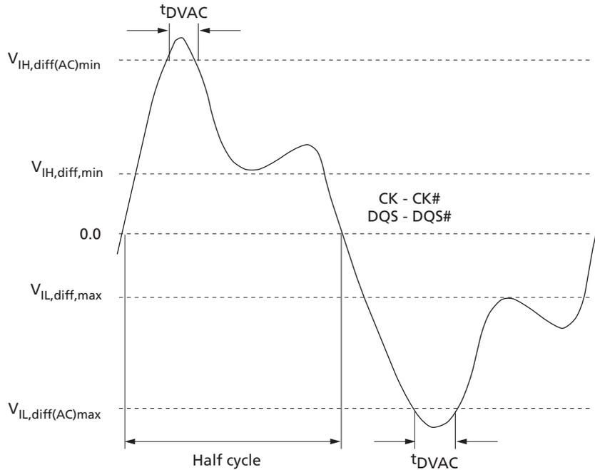
**Table 26: DDR3L 1.35V - Minimum Required Time  $t_{DVAC}$  for CK/CK#, DQS/DQS# Differential for AC Ringback**
