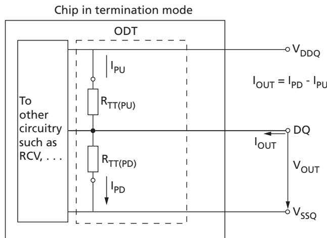
**Table 29: On-Die Termination DC Electrical Characteristics**
