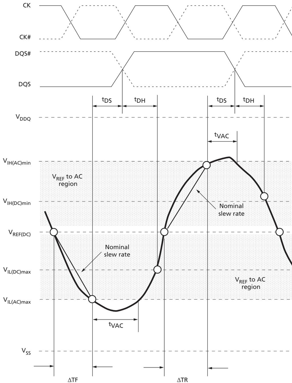
$$\text{Setup slew rate falling signal} = \frac{V_{REF(DC)} - V_{IL(AC)max}}{\Delta TF}$$
