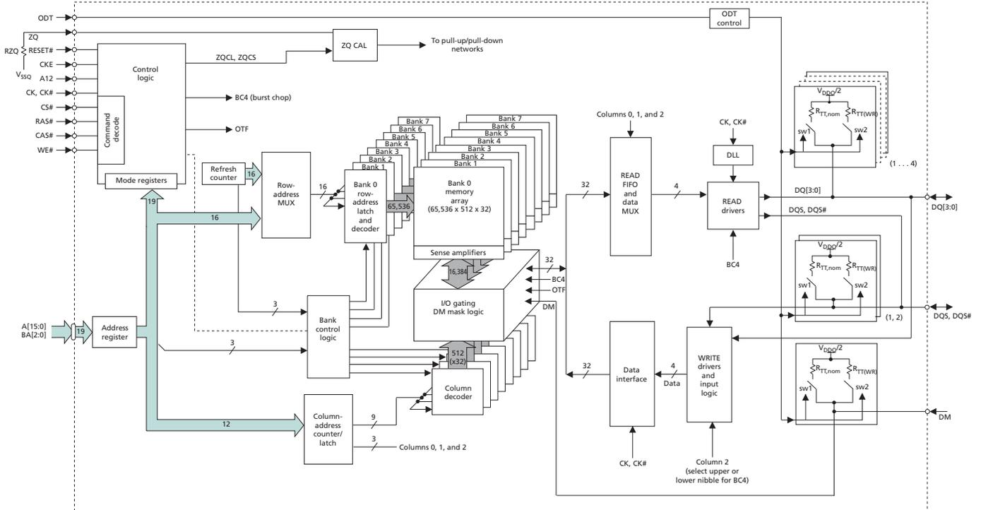
**Figure 4: 1 Gig x 8 Functional Block Diagram**
