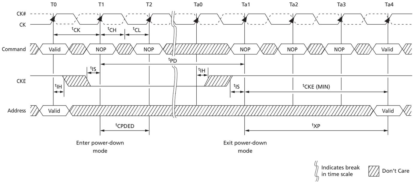
**Figure 95: Precharge Power-Down (Fast-Exit Mode) Entry and Exit**
