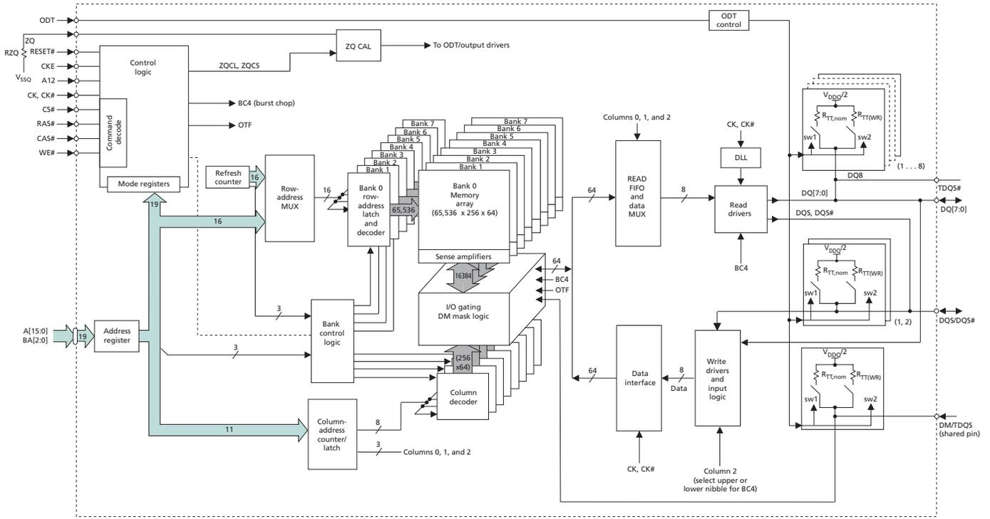
**Figure 5: 512 Meg x 16 Functional Block Diagram**
