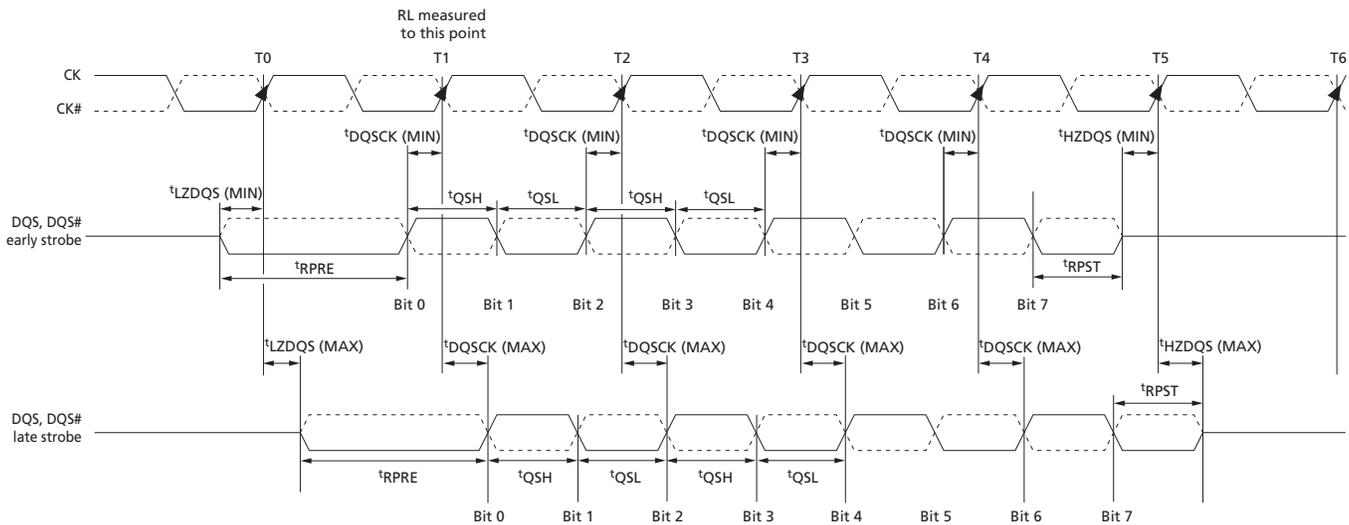
Figure 77: Method for Calculating  $t_{HZ}$  and  $t_{LZ}$
