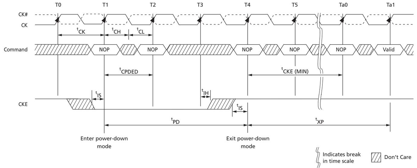
Figure 96: Precharge Power-Down (Slow-Exit Mode) Entry and Exit
