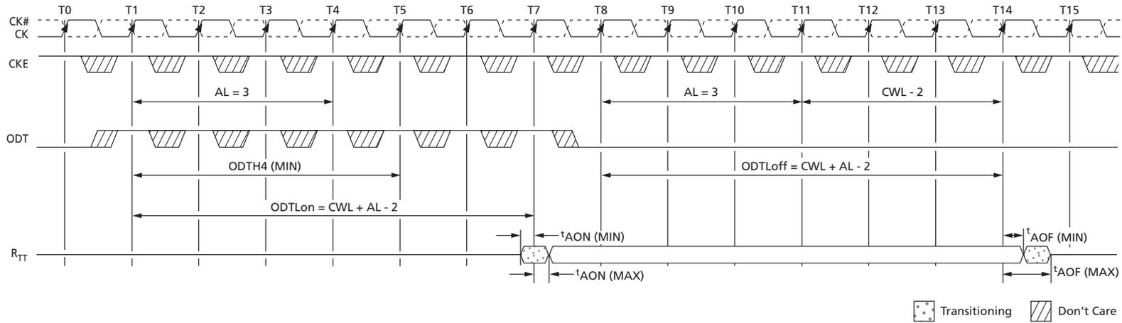
Note: 1. AL = 3; CWL = 5; ODTL<sub>on</sub> = WL = 6.0; ODTL<sub>off</sub> = WL - 2 = 6. R<sub>TT,nom</sub> is enabled.
