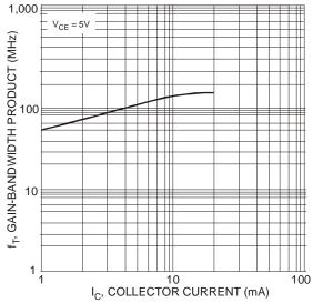
Fig. 5 Typical Gain-Bandwidth Product vs.
