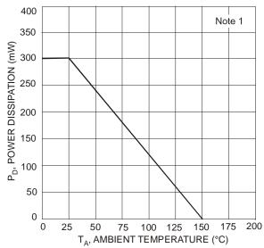
Fig. 1 Power Dissipation vs. Ambient Temperature
