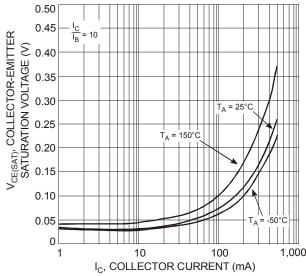
Figure 2 Collector-Emitter Saturation Voltage vs. Collector Current
