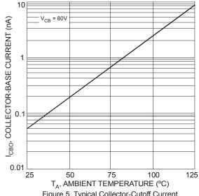
Figure 5 Typical Collector-Cutoff Current vs. Ambient Temperature
