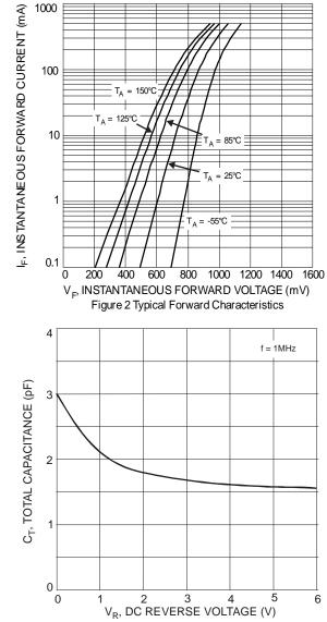
Figure 4 Total Capacitance vs. Reverse Voltage
