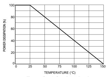
Figure 2. Steady State Power Derating
