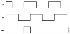
Figure 9. A, B, and NM Timing for Clockwise Rotation
