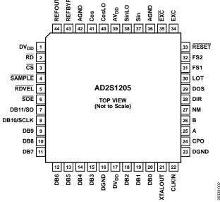
Figure 2. Pin Configuration
