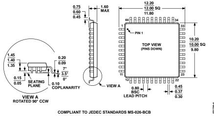
Figure 17. 44-Lead Low Profile Quad Flat Package [LQFP] (ST-44-1) Dimensions shown in millimeters
