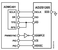
Figure 16. Connecting to the ADMC401
