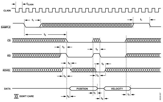
Figure 7. Parallel Port Read Timing
