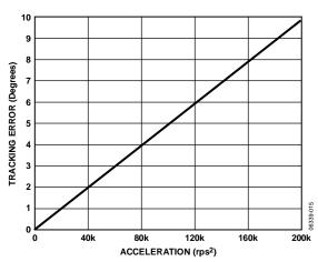
Figure 15. Tracking Error vs. Acceleration
