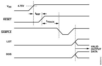
Figure 10. Power Supply Sequencing and Reset
