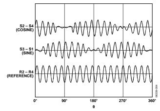
Figure 4. Electrical Resolver Representation
