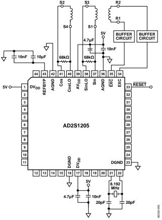
Figure 5. Connecting the AD2S1205 to a Resolver
