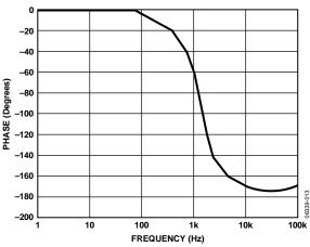
Figure 13. RDC System Phase Response
