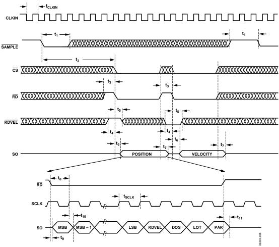
Figure 8. Serial Port Read Timing
