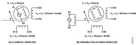
Figure 3. Classical Resolver vs. Variable Reluctance Resolver
