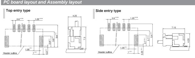
Note: 1. The above figure is the figure viewed from the connector mounting side. 2. Tolerances are non-cumulative: ±0.05 mm for all centers.
