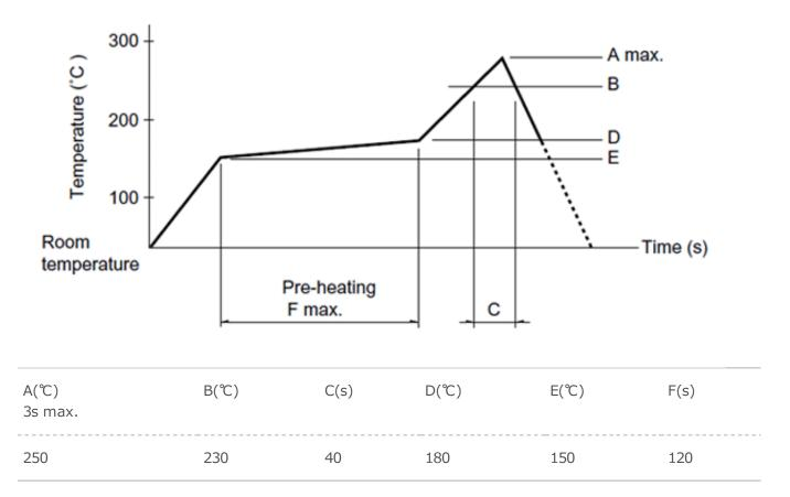
(1) The condition mentioned above is the temperature on the mounting surface of a PC board. There are cases where the PC board's temperature greatly differs from that of the switch, surface depending on the PC board's material, size, thickness, etc. The above-stated conditions shall also apply to switch surface temperatures.
