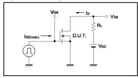
Fig.3-1 Switching Energy Measurement Circuit
