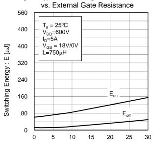
Fig.21 Typical Switching Loss
