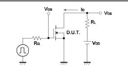
Fig.2-1 Gate Charge Measurement Circuit
