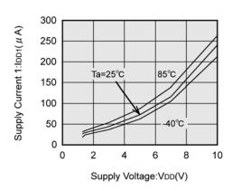
(7) Stand-By Current vs. Power Supply Voltage
