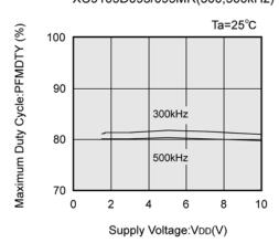
(24) PFM Duty Ratio vs. Power Supply Voltage
