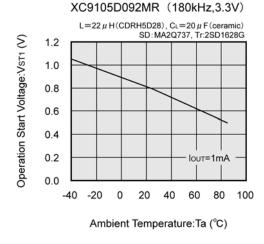
(19) Oscillation Start Voltage vs. Ambient Temperature
