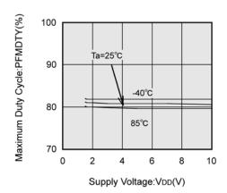
(10) PFM Duty Ratio vs. Power Supply Voltage
