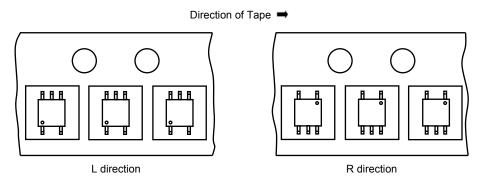
Figure 1 Device Orientation
