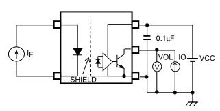
**TEST CIRCUIT 3: ICCL Test Circuit**
