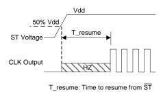
Figure 5. Standby Resume Timing (ST Mode Only)
