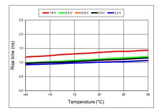
Figure 12. 20%-80% Rise Time vs Temperature
