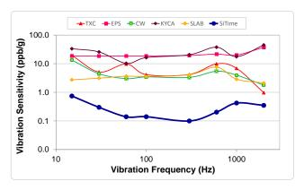
Figure 5. Vibration Robustness<sup>[5]</sup>
