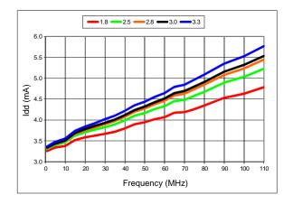
Figure 8. Idd vs Frequency
