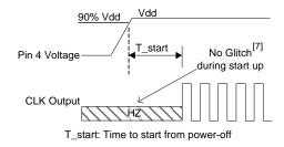
Figure 4. Startup Timing (OE/ST Mode)
