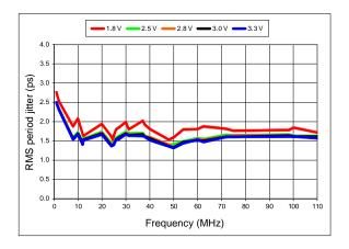
Figure 10. RMS Period Jitter vs Frequency
