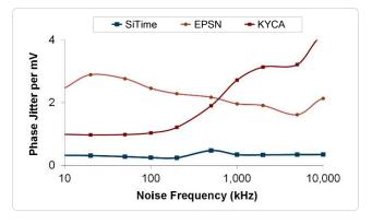
Figure 4. Power Supply Noise Rejection<sup>[4]</sup>
