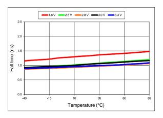
Figure 13. 20%-80% Fall Time vs Temperature
