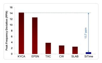
Figure 6. Shock Robustness<sup>[6]</sup>
