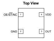
Figure 1. Pin Assignments
