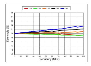
Figure 11. Duty Cycle vs Frequency
