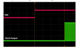
Figure 17. Startup Waveform vs. Vdd
