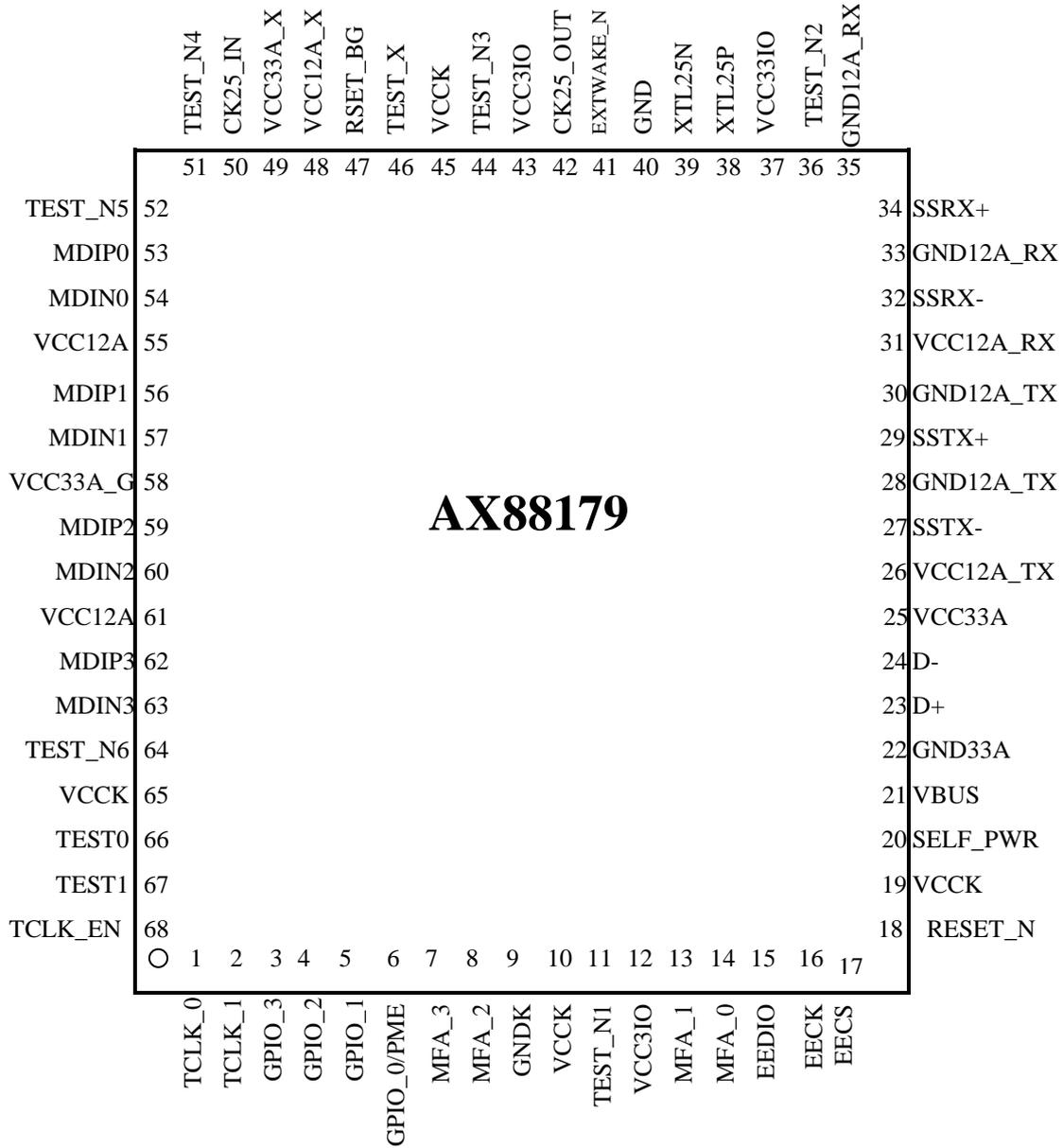
Figure 3 : Pinout Diagram
