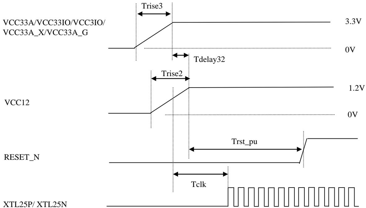
Note: The VCC12 includes VCCCK, VCC12A, and VCC12A\_X/TX/RX.
