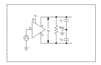
Figure 3 Driver Timing Test Circuit
