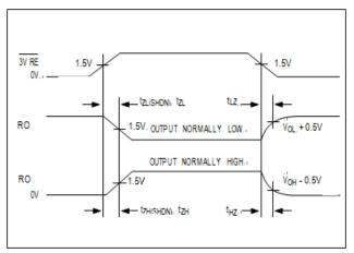
Figure 8. Receiver Enable and Disable Times
