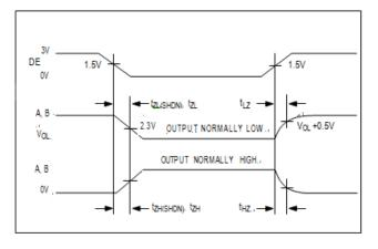
Figure 6. Driver Enable and Disable Times
