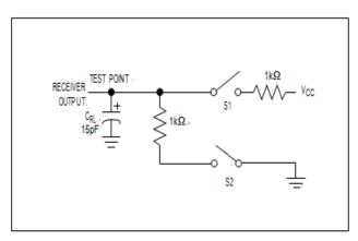
Figure 2. Receiver Enable/Disable Timing Test Load
