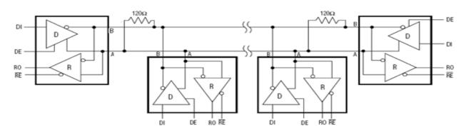
Figure 10 Typical Half-Duplex RS-485 Network
