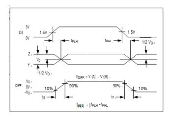
Figure 5 Driver Propagation Delays
