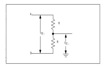
Figure 1. Driver DC Test Load
