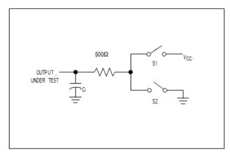
Figure 4 Driver Enable/Disable Timing Test Load
