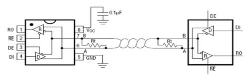
Figure 9 3085 Pin Configuration and Typical Half-Duplex Operating Circuit
