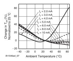
Fig. 7 - Turn-on Time vs. Temperature
