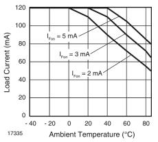
Fig. 1 - Recommended Operating Conditions
