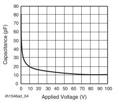
Fig. 5 - Switch Capacitance vs. Applied Voltage
