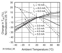
Fig. 8 - Turn-off Time vs. Temperature
