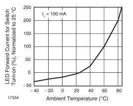
Fig. 3 - LED Current for Switch Turn-on vs. Temperature
