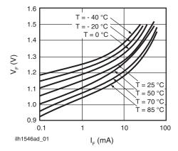
Fig. 2 - LED Voltage vs. Temperature
