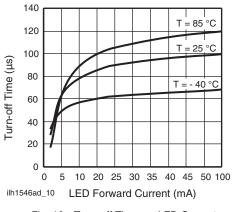
Fig. 10 - Turn-off Time vs. LED Current
