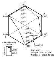
Test conditions: Shock is applied in  $\pm X$ ,  $\pm Y$ , and  $\pm Z$  directions three times each with and without energizing the Relays to check the number of contact malfunctions.
