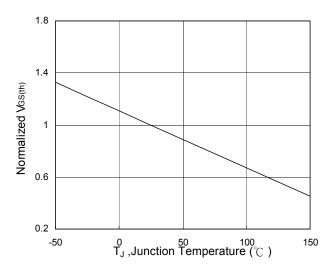
Fig.5 Normalized V<sub>GS(th)</sub> vs. T<sub>J</sub>
