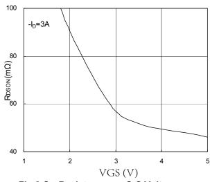
Fig.2 On-Resistance vs. G-S Voltage
