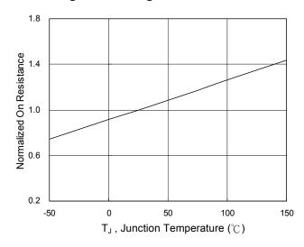
Fig.6 Normalized R<sub>DSON</sub> vs. T<sub>J</sub>
