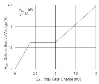
Fig.4 Gate-charge Characteristics
