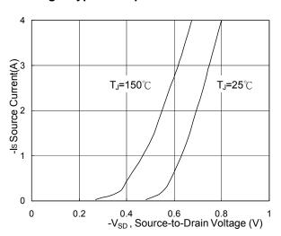
Fig.3 Forward Characteristics of Reverse
