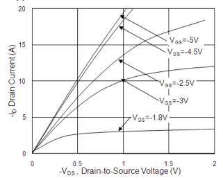
Fig.1 Typical Output Characteristics
