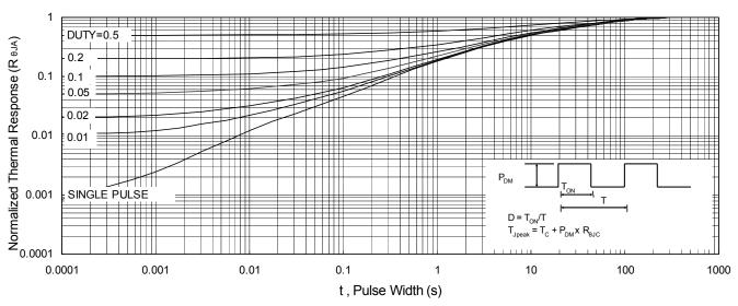
Fig.9 Normalized Maximum Transient Thermal Impedance
