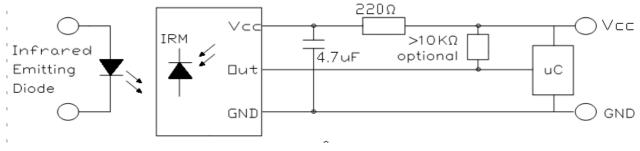
RC Filter should be connected closely between Vcc pin and GND pin.
