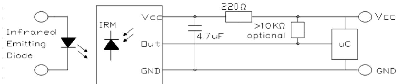
RC Filter should be connected closely between Vcc pin and GND pin.
