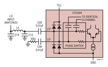
Figure 14. Recommended Single-Ended LO Input Configuration
