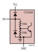
Figure 28. Simplified Schematic of the EN Pin Interface
