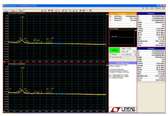
Figure 36.  $f_{RF}$  = 889MHz and 890MHz 2-Tone Receiver Test,  $f_{L0}$  = 881MHz. Ch.1 Is the I Channel and Ch.2 Is the Q Channel. Tested without LNA
