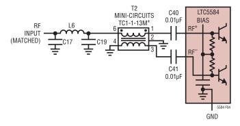
Figure 4: Simplified Schematic of the RF Interface
