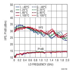
Figure 8. Broadband IIP3 and IP1dB
