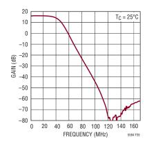
Figure 35. Baseband Gain Response without LNA
