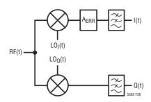
Figure 38. Signal Diagram for a Demodulator
