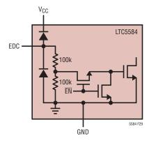
Figure 29. Simplified Schematic of the EDC Pin Interface core bias current and total power consumption for the chip. For example, adding  $487\Omega$  from the  $V_{BIAS}$  pin to GND will lower the DC current to 169mA, at the expense of reduced IIP3 performance. Figure 32 shows IIP3 and
