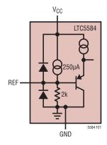
Figure 21. Simplified Schematic of the REF Pin Interface
