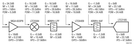
Figure 34. 900MHz Receiver Chain Analysis
