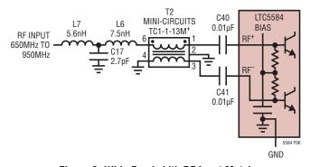
Figure 6. Wide Bandwidth RF Input Match
