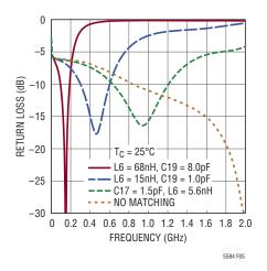
Figure 5. RF Input Return Loss
