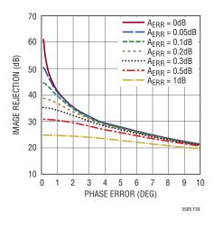
Figure 39. Image Rejection as a Function of Gain and Phase Errors
