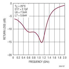
Figure 7. RF Input Return Loss for Wideband Match
