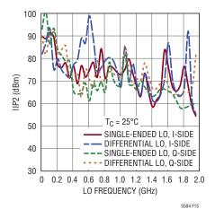
Figure 15. Broadband IIP2 with Differential and Single-Ended LO Drive
