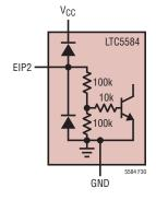
Figure 30. Simplified Schematic of the EIP2 Pin Interface
