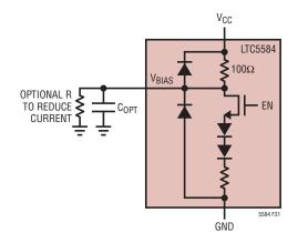
Figure 31. Simplified Schematic of the V<sub>BIAS</sub> Pin Interface
