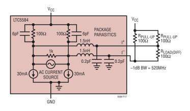
Figure 17. Simplified Model of the Baseband Output
