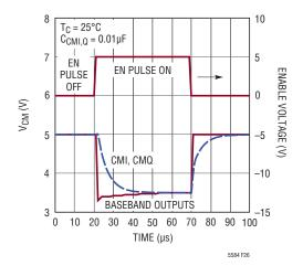
Figure 26. Common Mode Output Voltage with a Pulsed Enable
