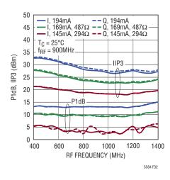
Figure 32. IIP3 and P1dB vs DC Current and V<sub>BIAS</sub> Resistor Value
