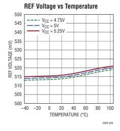
**TYPICAL PERFORMANCE CHARACTERISTICS** 140MHz application.  $V_{CC} = 5V$ , EN = 5V, EDC = 0V, EIP2 = 0V, REF = 0.5V,  $T_C = 25^{\circ}C$ ,  $P_{L0} = 6dBm$ ,  $f_{L0} = 130MHz$ ,  $f_{RF1} = 140MHz$ ,  $f_{RF2} = 141MHz$ ,  $f_{BB} = 10MHz$ ,  $P_{RF1} = P_{RF2} = -5dBm$ , DC Blocks and Mini-Circuits PSCJ-2-1 180° combiner at baseband outputs de-embedded from measurement unless otherwise noted. Test circuit with RF and LO ports impedance matched as in Figure 1.
