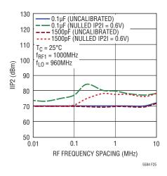
Figure 25. IIP2 vs Common Mode Decoupling Capacitance
