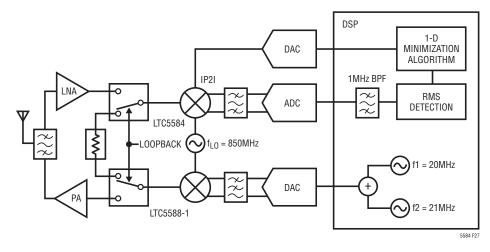
Figure 27. Block Diagram for a Direct Conversion Transceiver with IM2 Adjustment. Only the I-Channel Is Shown
