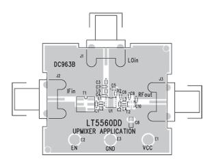
Figure 23. Upconverting Mixer Evaluation Board (DC963B)—See Table 1
