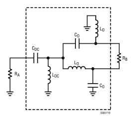
Figure 19. Lumped Element Balun
