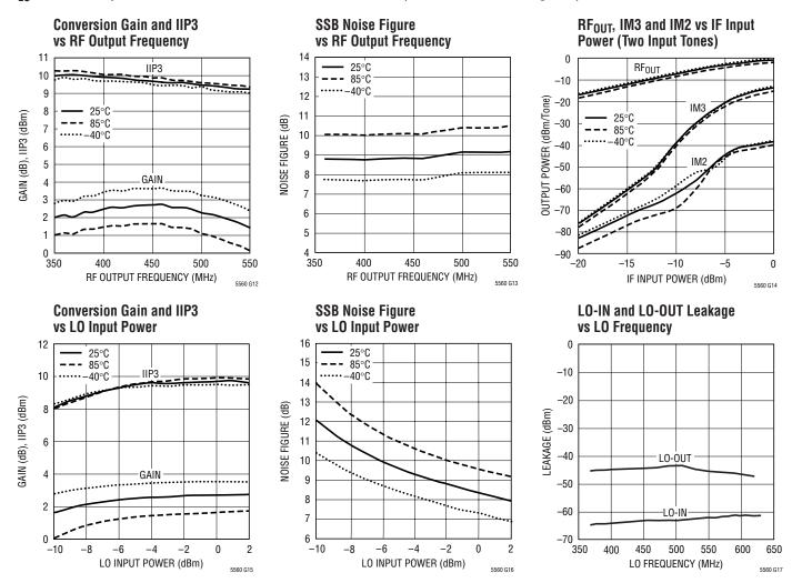
1900MHz Upconverting Mixer Application:  $V_{CC}$  = 3V,  $I_{CC}$  = 10mA, EN = 3V,  $T_A$  = 25°C,  $f_{IN}$  = 140MHz,  $P_{IN}$  = -20dBm (-20dBm/tone for 2-tone IIP3 tests,  $\Delta f$  = 1MHz),  $f_{LO}$  = 1760MHz,  $P_{LO}$  = -2dBm, output measured at 1900MHz, unless otherwise noted. (Test circuit shown in Figure 1)
