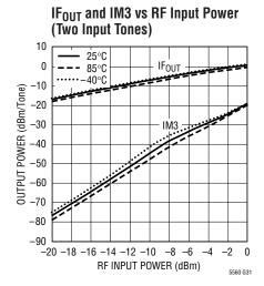
450MHz Downconverting Mixer Application:  $V_{CC} = 3V$ ,  $I_{CC} = 10mA$ , EN = 3V,  $T_A = 25^{\circ}C$ ,  $f_{IN} = 450MHz$ ,  $P_{IN} = -20dBm$  (-20dBm/tone for 2-tone IIP3 tests,  $\Delta f = 1MHz$ ),  $f_{LO} = 520MHz$ ,  $P_{LO} = -2dBm$ , output measured at 70MHz, unless otherwise noted. (Test circuit shown in Figure 3)
