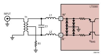
Figure 4. Input Port with Lowpass External Matching Topology
