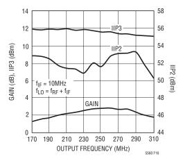
Figure 16. LT5560 Performance in 240MHz Upconverting Mixer Application
