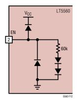
Figure 12. Enable Input Circuit
