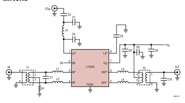
Component Values for  $f_{OUT} = 900 MHz, \, f_{IN} = 140 MHz \, and \, f_{LO} = 760 MHz$
