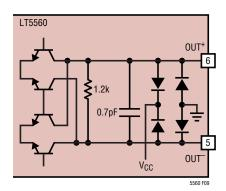
Figure 9. Output Port Schematic
