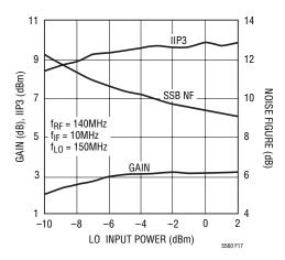
Figure 17. LT5560 Performance in 140MHz Downconverting Mixer Application
