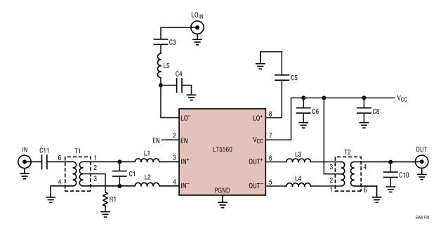
Upconverting Mixer Component Values for  $f_{\text{IN}}$  = 70MHz,  $f_{\text{OUT}}$  = 450MHz and  $f_{\text{LO}}$  = 520MHz
