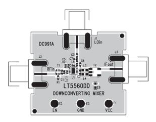
Figure 24. Downconverting Mixer Evaluation Board (DC991A)—See Table 1
