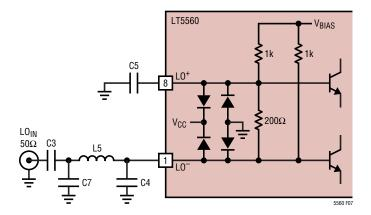
Figure 7. LO Input Schematic
