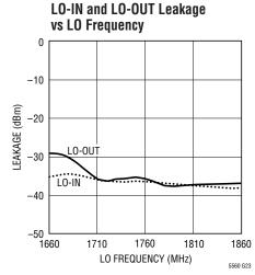
900MHz Downconverting Mixer Application:  $V_{CC}$  = 3V,  $I_{CC}$  = 10mA, EN = 3V,  $T_A$  = 25°C,  $f_{IN}$  = 900MHz,  $P_{IN}$  = -20dBm (-20dBm/tone for 2-tone IIP3 tests,  $\Delta f$  = 1MHz),  $f_{LO}$  = 760MHz,  $P_{LO}$  = -2dBm, output measured at 140MHz, unless otherwise noted. (Test circuit shown in Figure 2)
