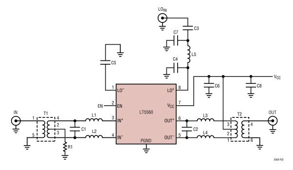
Component Values for  $f_{\text{IN}} = 900 \text{MHz}, \, f_{\text{OUT}} = 140 \text{MHz}$  and  $f_{\text{LO}} = 760 \text{MHz}$
