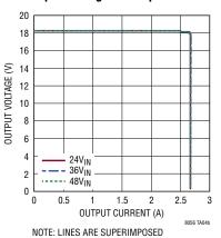
Two LTM8056s Paralleled to Get More Output Current. The Two µModules Are Synchronized and Switching 180° Out Of Phase
