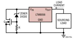
Figure 5a. The MOSFET Q Dissipates Momentary Energy to GND. The Zener Diode and Resistor Are Chosen to Ensure That the MOSFET Turns On Above the Maximum  $V_{\text{IN}}$  Voltage Under Normal Operation
