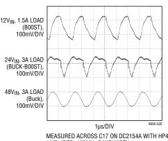
MEASURED ACROSS C17 ON DC2154A WITH HP461 AMPLIFIER, 150MHz BANDWIDTH
