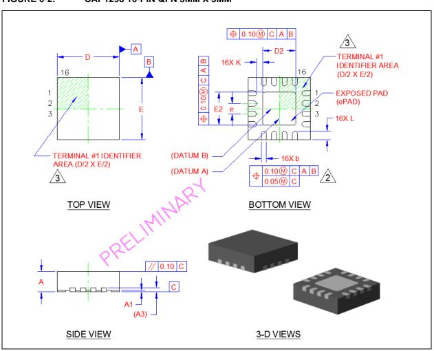
FIGURE 6-2: CAP1298 16-PIN QFN 3MM X 3MM
