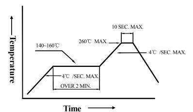
3). DIP soldering (Wave Soldering):
