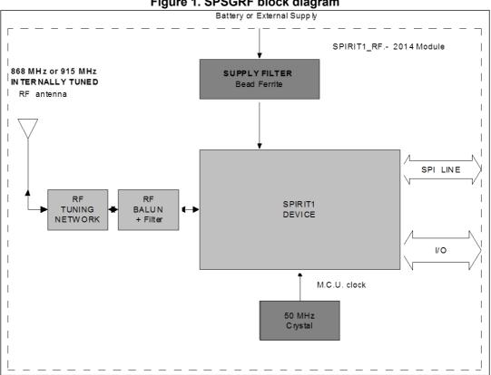
Figure 1. SPSGRF block diagram
