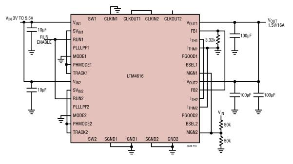
Figure 19. LTM4616 Two Outputs Parallel, 1.5V at 16A Design
