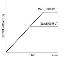
Figure 6. Output Voltage Coincident Tracking
