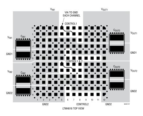
Figure 17. Recommended PCB Layout (LGA and BGA PCB Layouts Are Identical with the Exception of Circle Pads for BGA. See Package Description.)
