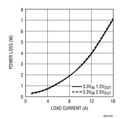
Figure 7. 1.2V, 2.5V Power Loss
