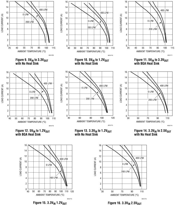
Figure 15. 3.3  $V_{IN}$  1.2  $V_{OUT}$  with BGA Heat Sink
