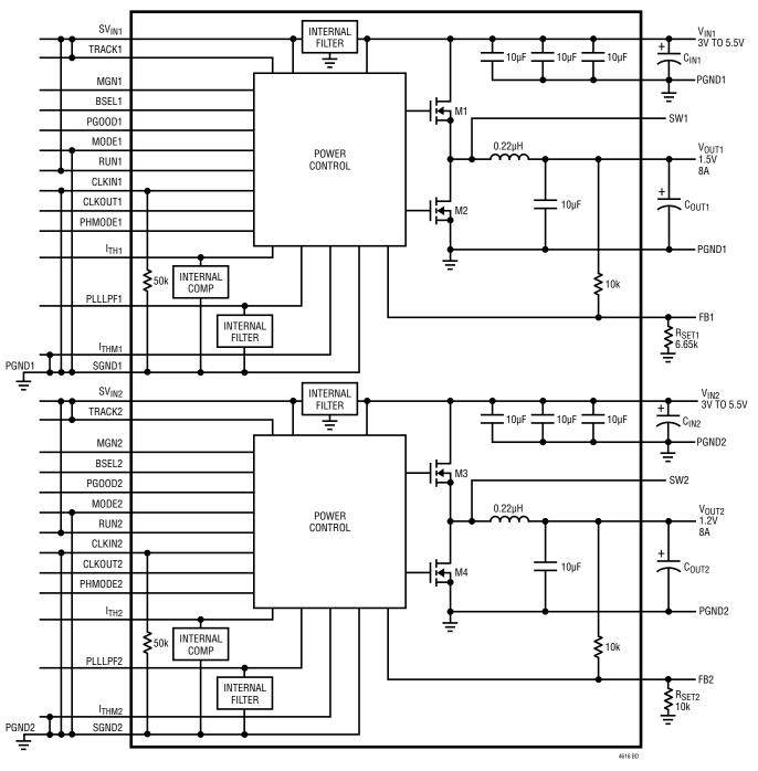
Figure 1. Simplified LTM4616 Block Diagram
