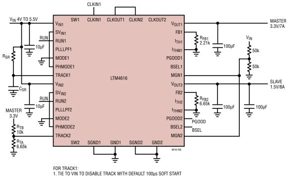
2. APPLY A CONTROL RAMP WITH  $R_{SR}$  AND  $C_{SR}$  TIED TO  $V_{IN}$  WITH  $t = -(In(1-0.596/V_{IN}) \cdot R_{SR} \cdot C_{SR}))$
