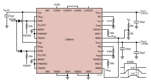
Figure 20. LTM4616 Output Sequencing Application
