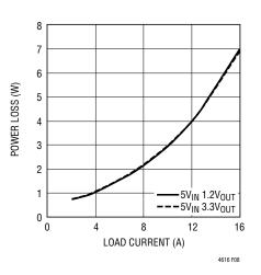
Figure 8. 1.2V, 3.3V Power Loss
