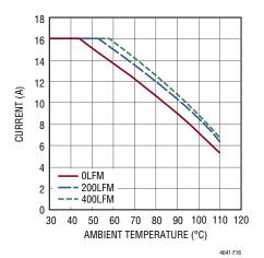
Figure 16. 5V<sub>IN</sub> to 1.0V<sub>OUT</sub> Derating Curve 4-Channel Paralleled, No Heat Sink
