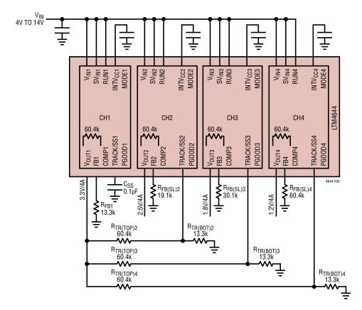
Figure 5. Output Ratiometric Tracking Schematic
