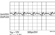
V<sub>OUT</sub> = 1.5V INPUT CAPACITOR = 22µF SANYO ELECTROLYTIC CAPACITOR (OPTIONAL) + 2× 22µF CERAMIC CAP. OUTPUT CAPACITOR = 2× 47µF CERAMIC CAP. SOFT-START CAPACITOR = 0.1µF 20MHz MEASUREMENT BANDWIDTH
