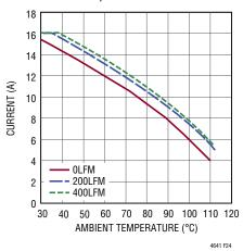
Figure 24. 5V<sub>IN</sub> to 3.3V<sub>OUT</sub> Derating Curve 4-Channel Paralleled, No Heat Sink
