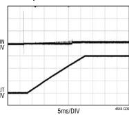
$V_{\text{IN}} = 12\text{V}, V_{\text{OUT}} = 1.5\text{V} \\ \text{INPUT CAPACITOR} = 150\mu\text{F SANYO ELECTROLYTIC} \\ \text{CAPACITOR (OPTIONAL)} + 22\mu\text{F CERAMIC CAPACITOR} \\ \text{OUTPUT CAPACITOR} = 47\mu\text{F CERAMIC CAPACITOR} \\ \text{SOFT-START CAPACITOR} = 0.1\mu\text{F} \\ \\$
