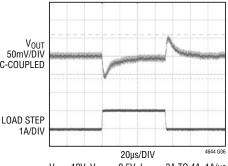
$V_{IN} = 12V$ ,  $V_{OUT} = 2.5V$ ,  $I_{OUT} = 3A TO 4A$ ,  $1A/\mu s$ OUTPUT CAPACITOR = 1 • 47μF CERAMIC
