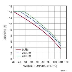
Figure 17. 12V<sub>IN</sub> to 1.0V<sub>OUT</sub> Derating Curve 4-Channel Paralleled, No Heat Sink
