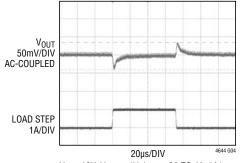
$V_{IN} = 12V$ ,  $V_{OUT} = 1V$ ,  $I_{OUT} = 3A TO 4A$ ,  $1A/\mu s$ OUTPUT CAPACITOR = 1 • 47μF CERAMIC
