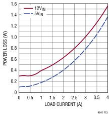
Figure 13. Power Loss at 2.5V Output, (Each Channel, 25°C)
