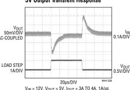
V<sub>IN</sub> = 12V, V<sub>OUT</sub> = 5V, I<sub>OUT</sub> = 3A TO 4A, 1A/µs OUTPUT CAPACITOR = 47µF CERAMIC
