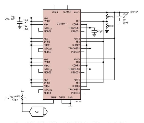
Figure 36. 4V to 14V Input, 4-Phase, 1.2V at 16A Design with Temperature Monitoring
