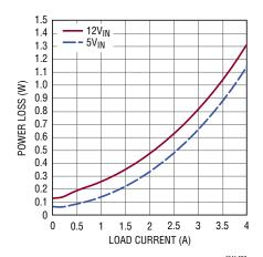
Figure 9. Power Loss at 1.0V Output, (Each Channel, 25°C)
