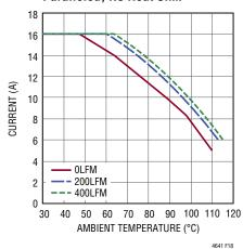
Figure 18. 5V<sub>IN</sub> to 1.0V<sub>OUT</sub> Derating Curve 4-Channel Paralleled, BGA Heat Sink
