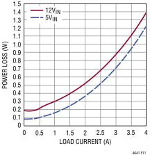
Figure 11. Power Loss at 1.5V Output, (Each Channel, 25°C)
