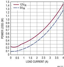
Figure 12. Power Loss at 1.8V Output, (Each Channel, 25°C)
