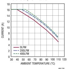
Figure 20. 5V<sub>IN</sub> to 1.5V<sub>OUT</sub> Derating Curve 4-Channel Paralleled, No Heat Sink
