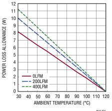
Figure 31. Power Loss Allowance vs. Ambient Temperature BGA Heat Sink
