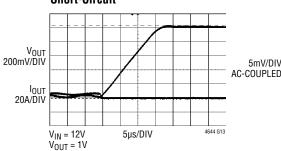
INPUT CAPACITOR = 22µF SANYO ELECTROLYTIC CAPACITOR (OPTIONAL) + 2× 22µF CERAMIC CAP. OUTPUT CAPACITOR = 2× 47µF CERAMIC CAP. SOFT-START CAPACITOR = 0.1µF
