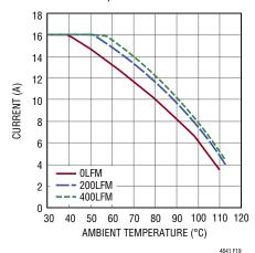
Figure 19. 12V<sub>IN</sub> to 1.0V<sub>OUT</sub> Derating Curve 4-Channel Paralleled, BGA Heat Sink
