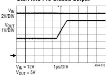
INPUT CAPACITOR = 22µF SANYO ELECTROLYTIC CAPACITOR (OPTIONAL) + 2× 22µF CERAMIC CAP. OUTPUT CAPACITOR = 2× 47µF CERAMIC CAP. SOFT-START CAPACITOR = 0.1µF
