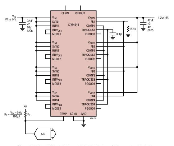
Figure 35. 4V to 14V Input, 4-Phase, 1.2V at 16A Design with Temperature Monitoring
