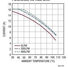
Figure 26. 5V<sub>IN</sub> to 3.3V<sub>OUT</sub> Derating Curve 4-Channel Paralleled, BGA Heat Sink
