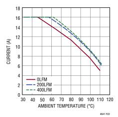
Figure 22. 5V<sub>IN</sub> to 1.5V<sub>OUT</sub> Derating Curve 4-Channel Paralleled, BGA Heat Sink
