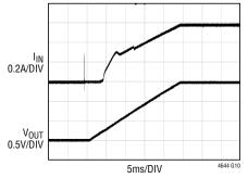
$V_{\text{IN}} = 12V, V_{\text{OUT}} = 1.5V$ INPUT CAPACITOR =  $150\mu\text{F}$  SANYO ELECTROLYTIC CAPACITOR (OPTIONAL) +  $22\mu\text{F}$  CERAMIC CAPACITOR OUTPUT CAPACITOR =  $47\mu\text{F}$  CERAMIC CAPACITOR SOFT-START CAPACITOR =  $0.1\mu\text{F}$
