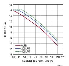
Figure 21. 12V<sub>IN</sub> to 1.5V<sub>OUT</sub> Derating Curve 4-Channel Paralleled, No Heat Sink
