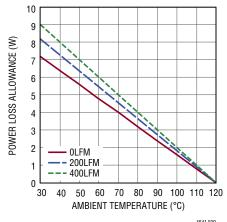
Figure 30. Power Loss Allowance vs. Ambient Temperature No Heat Sink
