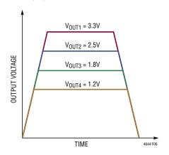
Figure 6. Output Coincident Tracking Waveform
