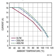
Figure 23. 12V<sub>IN</sub> to 1.5V<sub>OUT</sub> Derating Curve 4-Channel Paralleled, BGA Heat Sink
