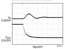
$\begin{array}{l} V_{IN}=12V,\,V_{OUT}=1.5V\\ INPUT \,CAPACITOR=150\mu F\,SANYO\,ELECTROLYTIC\\ CAPACITOR\,(OPTIONAL)+22\mu F\,CERAMIC\,CAPACITOR\\ OUTPUT\,CAPACITOR=47\mu F\,CERAMIC\,CAPACITOR \end{array}$
