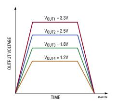
Figure 4. Output Ratiometric Tracking Waveform
