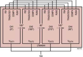
Figure 2. 2+2 and 4 Channels Parallel Concept Schematic
