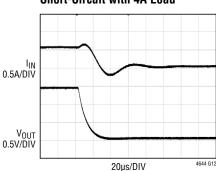
$V_{\rm IN}$  = 12V,  $V_{\rm OUT}$  = 1.5V INPUT CAPACITOR = 150 $\mu$ F SANYO ELECTROLYTIC CAPACITOR (OPTIONAL) + 22 $\mu$ F CERAMIC CAPACITOR OUTPUT CAPACITOR = 47 $\mu$ F CERAMIC CAPACITOR
