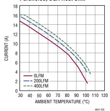
Figure 25. 12V<sub>IN</sub> to 3.3V<sub>OUT</sub> Derating Curve 4-Channel Paralleled, No Heat Sink
