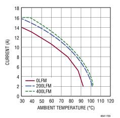
Figure 27. 12V<sub>IN</sub> to 3.3V<sub>OUT</sub> Derating Curve 4-Channel Paralleled, BGA Heat Sink
