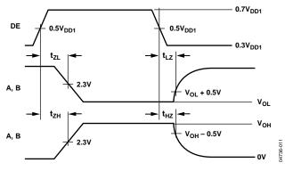
Figure 11. Driver Enable/Disable Timing
