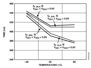
Figure 19. Driver Propagation Delay vs. Temperature
