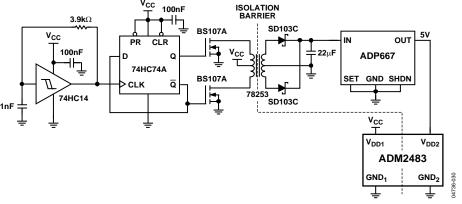
Figure 30. Isolated Power Supply Circuit
