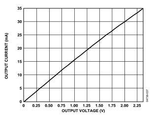
Figure 25. Output Current vs. Receiver Output Low Voltage
