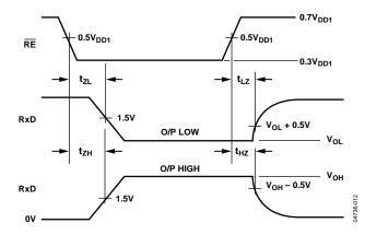
Figure 12. Receiver Enable/Disable Timing
