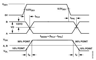
Figure 9. Driver Propagation Delay, Rise/Fall Timing
