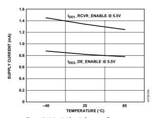
Figure 13. Unloaded Supply Current vs. Temperature
