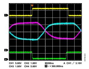
Figure 22. Driver/Receiver Propagation Delay Low to High
