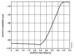
Figure 15. Output Current vs. Driver Output High Voltage
