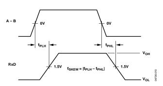
Figure 10. Receiver Propagation Delay
