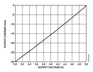
Figure 24. Output Current vs. Receiver Output High Voltage
