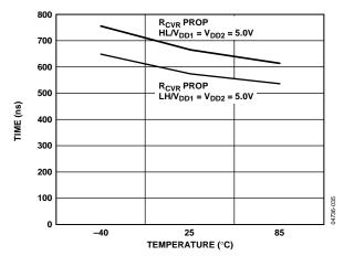
Figure 20. Receiver Propagation Delay vs. Temperature
