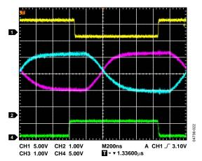
Figure 21. Driver/Receiver Propagation Delay High to Low
