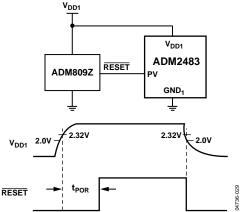
Figure 29. Driving PV with ADM809Z
