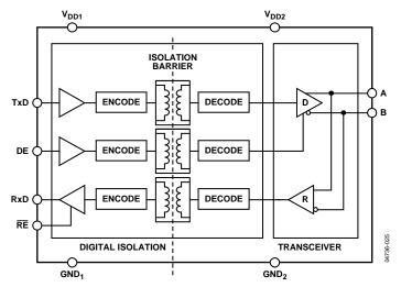
Figure 26. ADM2483 Digital Isolation and Transceiver Sections
