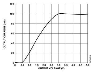
Figure 14. Output Current vs. Driver Output Low Voltage
