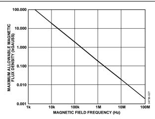
Figure 27. Maximum Allowable External Magnetic Flux Density
