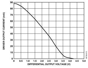
Figure 18. Driver Output Current vs. Differential Output Voltage
