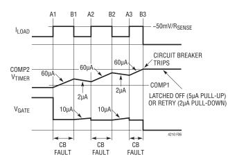
Figure 6. Multiple Intermittent Overcurrent Condition
