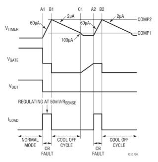
Figure 8. Automatic Retry After Overcurrent Fault
