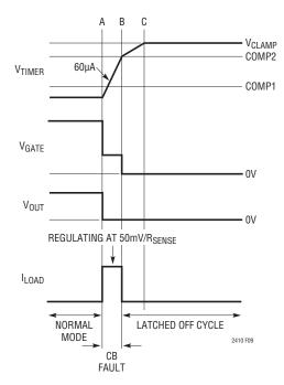
Figure 9. Latchoff After Overcurrent Fault
