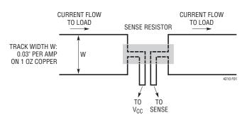
Figure 1. Making PCB Connections to the Sense Resistor
