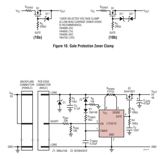
Figure 11. Supply Side Overvoltage Protection
