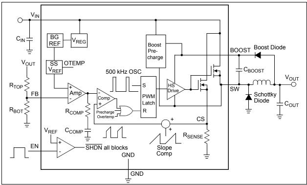
FIGURE 4-1: MCP16301/H Block Diagram.
