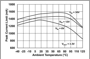
**FIGURE 2-10:** Peak Current Limit vs. Temperature;  $V_{OUT} = 3.3V$ .
