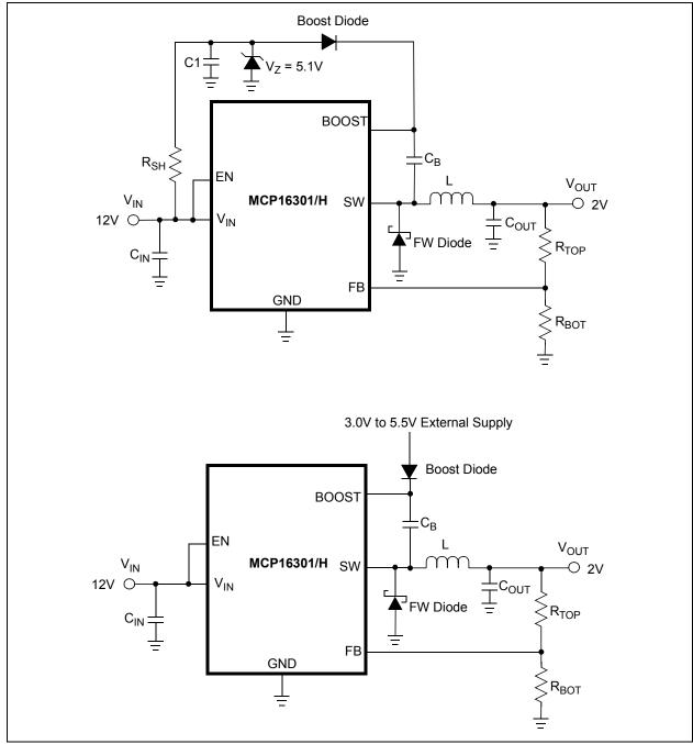
FIGURE 4-3: Shunt and External Boost Supply.
