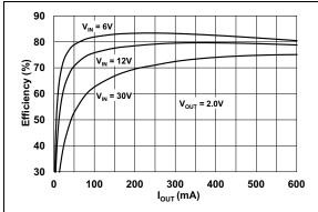
FIGURE 2-1: 2.0V V<sub>OUT</sub> Efficiency vs. I<sub>OUT</sub>.
