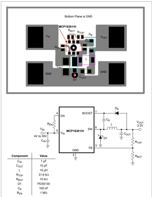
FIGURE 5-2: MCP16301/H SOT-23-6 D<sup>2</sup> Recommended Layout, 200 mA Design.
