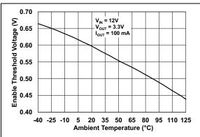
**FIGURE 2-14:** EN Threshold Voltage vs. Temperature.
