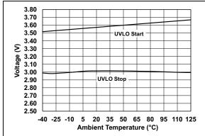
FIGURE 2-13: Undervoltage Lockout vs. Temperature.
