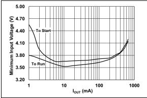
FIGURE 2-17: Typical Minimum Input Voltage vs. Output Current.
