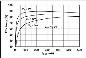
**FIGURE 2-2:** 3.3V  $V_{OUT}$  Efficiency vs.  $I_{OUT}$
