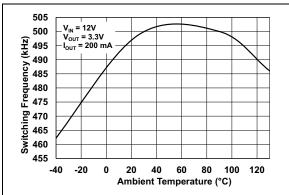
**FIGURE 2-8:** Switching Frequency vs. Temperature;  $V_{OUT} = 3.3V$ .
