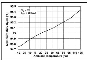
**FIGURE 2-9:** Maximum Duty Cycle vs. Ambient Temperature;  $V_{OUT} = 5.0V$ .
