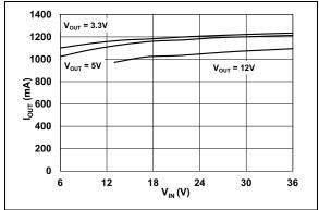
**FIGURE 2-6:** Maximum Output Current vs. V<sub>IN</sub>.
