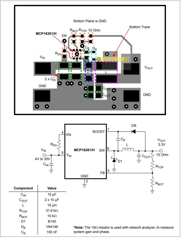
FIGURE 5-1: MCP16301/H SOT-23-6 Recommended Layout, 600 mA Design.
