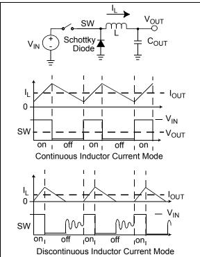
FIGURE 4-2: Step-Down Converter.
