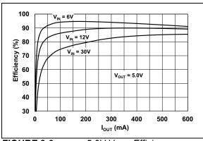
FIGURE 2-3: 5.0V V<sub>OUT</sub> Efficiency vs. I<sub>OUT</sub>.
