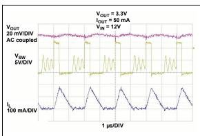
FIGURE 2-15: Light Load Switching Waveforms.
