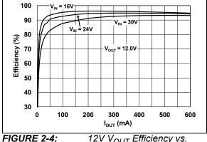
FIGURE 2-4: 12V V<sub>OUT</sub> Efficiency vs. I<sub>OUT</sub>
