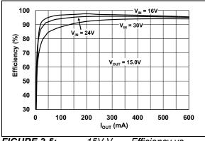
FIGURE 2-5: 15V V<sub>OUT</sub> Efficiency vs. I<sub>OUT</sub>.
