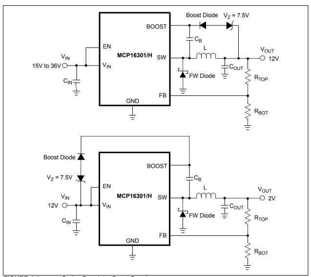
FIGURE 4-4: Series Regulator Boost Supply.
