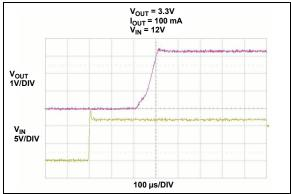
**FIGURE 2-19:** Start-Up from  $V_{IN}$ .
