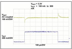
FIGURE 2-20: Load Transient Response.
