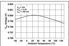
FIGURE 2-12:  $V_{FB}$  vs. Temperature;  $V_{OUT} = 3.3V$ .
