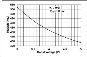
FIGURE 2-11: Switch R<sub>DSON</sub> vs. V<sub>BOOST</sub>.
