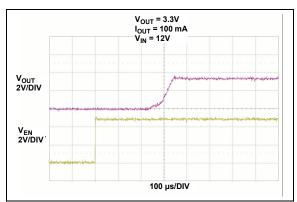
FIGURE 2-18: Start-Up From Enable.
