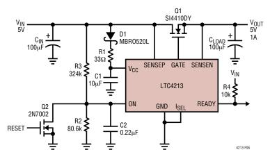
Figure 6. Single Supply Electronic Fuse
