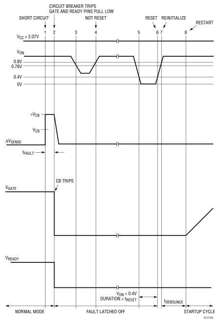
Figure 3. Resetting Fault Timing Diagram
