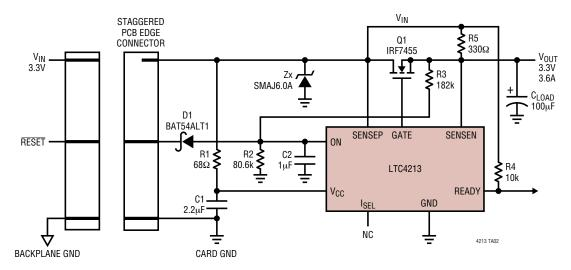
Figure 7. Single Supply Hot Board Insertion
