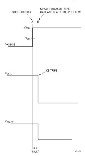
Figure 2. Short Circuit Fault Timing Diagram
