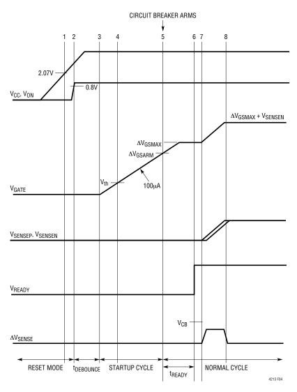
Figure 4. Load Supply Power-Up After Circuit Breaker Armed
