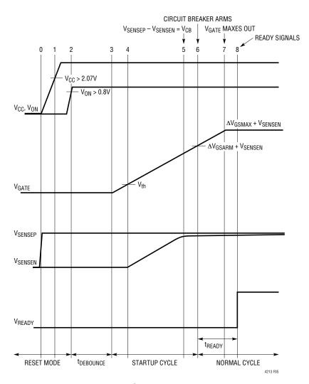
Figure 5. Load Supply Power-Up Before V<sub>CC</sub>
