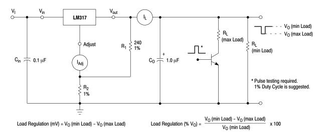
Figure 4. Load Regulation and  $\Delta I_{\mbox{Adj}}\mbox{/Load}$  Test Circuit
