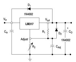
Figure 20. Voltage Regulator with Protection Diodes
