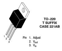
Heatsink surface connected to Pin 2.
