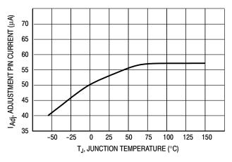
Figure 9. Adjustment Pin Current
