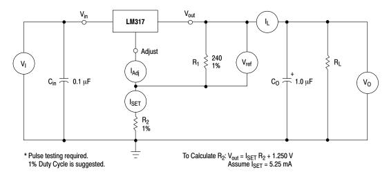
Figure 5. Standard Test Circuit
