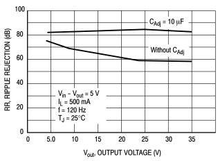
Figure 13. Ripple Rejection versus Output Voltage
