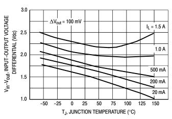
Figure 10. Dropout Voltage
