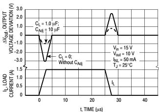
Figure 18. Load Transient Response
