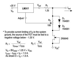
Figure 23. Adjustable Current Limiter
