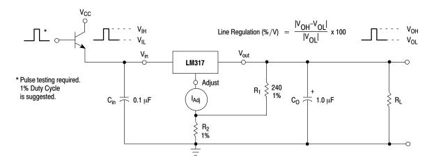
Figure 3. Line Regulation and  $\Delta I_{\mbox{Adj}}/\mbox{Line}$  Test Circuit
