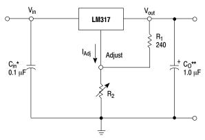
$^{\star}$  C<sub>in</sub> is required if regulator is located an appreciable distance from power supply filter.
