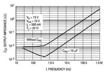
Figure 16. Output Impedance
