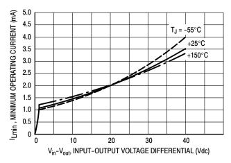
Figure 12. Minimum Operating Current
