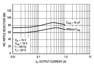
Figure 14. Ripple Rejection versus
