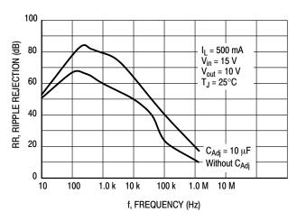
Figure 15. Ripple Rejection versus Frequency
