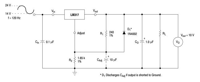
Figure 6. Ripple Rejection Test Circuit
