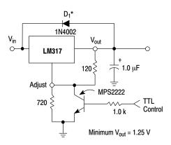
$^{\star}$  D<sub>1</sub> protects the device during an input short circuit.
