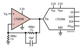
Figure 3. Single Supply 12-Bit ADC Driver
