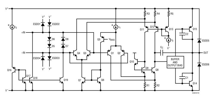
Figure 1. LTC6246/LTC6247/LTC6248 Simplified Schematic Diagram
