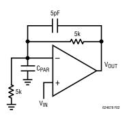
Figure 2. 5pF Feedback Cancels Parasitic Pole
