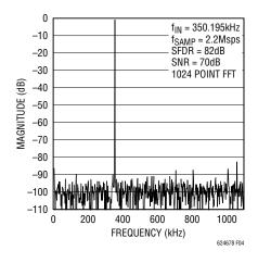
Figure 4. 350kHz FFT Showing 82dB SFDR
