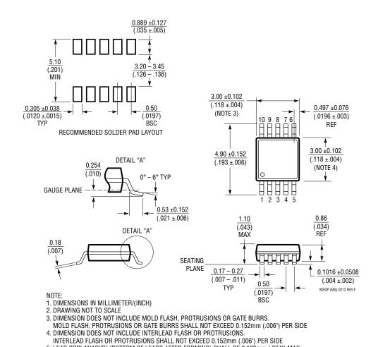
5. LEAD COPLANARITY (BOTTOM OF LEADS AFTER FORMING) SHALL BE 0.102mm (.004") MAX
