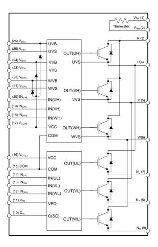
Figure 3. Internal Block Diagram
