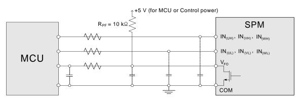
Figure 14. Recommended MCU I/O Interface Circuit
