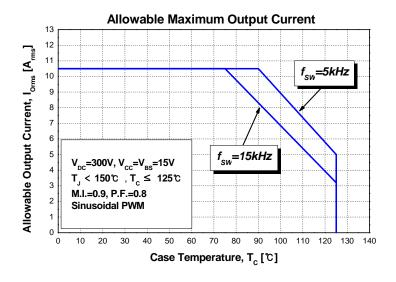
Figure 8. Allowable Maximum Output Current
