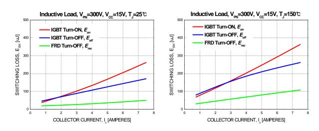
Figure 5. Switching Loss Characteristics (Typical)
