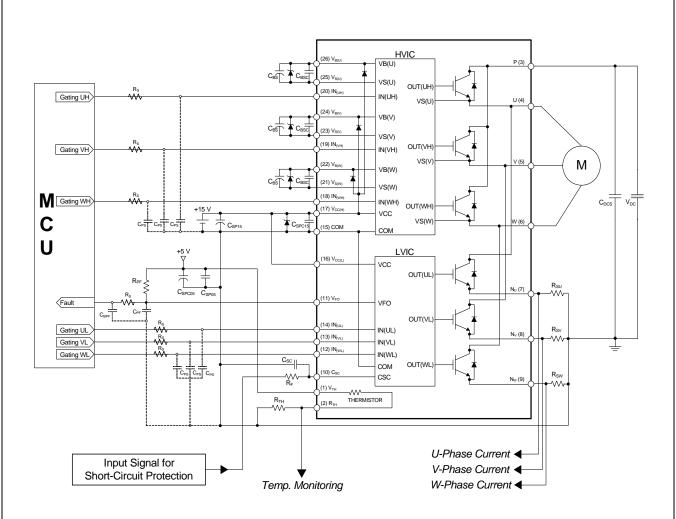
**Figure 15. Typical Application Circuit**
