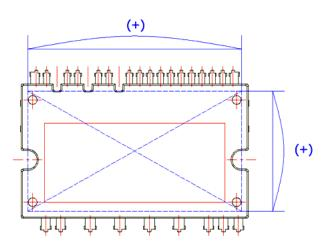
Figure 9. Flatness Measurement Position
