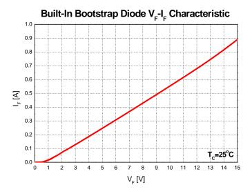
Figure 7. Built-In Bootstrap Diode Characteristic
