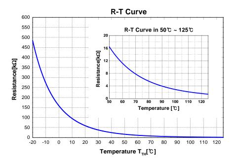
Figure. 6. R-T Curve of The Built-In Thermistor
