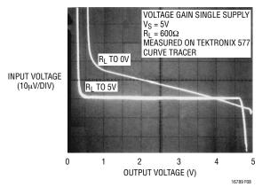
Figure 8. Voltage Gain Single Supply
