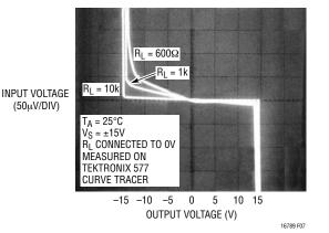
Figure 7. Voltage Gain Split Supply
