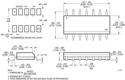
MOLD FLASH OR PROTRUSIONS SHALL NOT EXCEED .006" (0.15mm)
