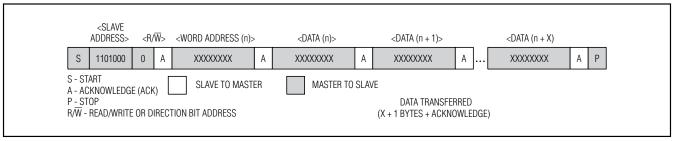
Figure 3. Data Write—Slave Receiver Mode
