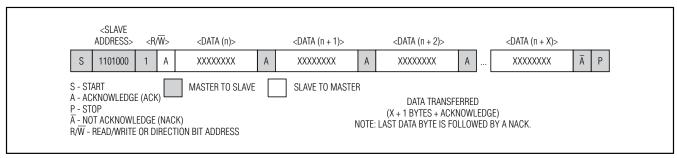
Figure 4. Data Read—Slave Transmitter Mode
