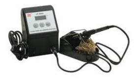
The Xytronic LF-3200 120W Digital Soldering Station has a digital temperature readout and a soldering temperature range of 200 to 500°C. Its high power and high frequency electronic circuitry maintains the soldering temperature within 3°C by means of a temperature sensor mounted in the head of the heating element which is in close contact with the actual soldering tip of the soldering iron.
