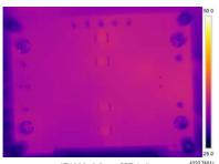
LT4320+2.5m $\Omega$  FET (×4) CONDITIONS: 24V AC<sub>IN</sub>, 9.75A DC LOAD ON SAME PCB
