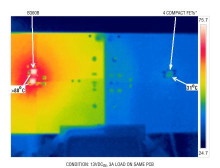
Figure 3. Thermograph: B360B vs LT4320 +4 Compact FETs
