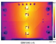
Thermograph of LT4320 Driving Four MOSFETs
