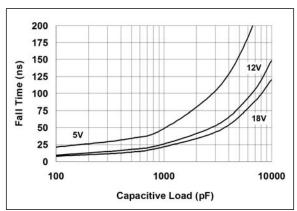
FIGURE 2-5: Fall Time vs. Capacitive Load.
