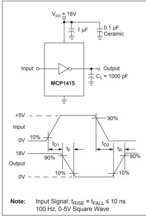
FIGURE 4-1: Inverting Driver Timing Waveform.
