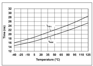
**FIGURE 2-3:** Rise and Fall Times vs. Temperature.
