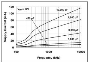
FIGURE 2-17: Supply Current vs. Frequency.
