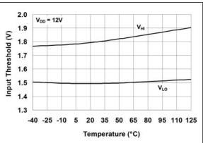
FIGURE 2-12: Input Threshold vs. Temperature.
