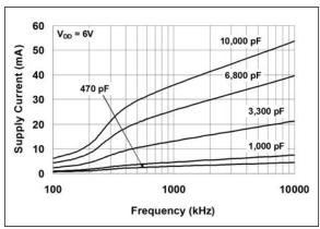
FIGURE 2-18: Supply Current vs. Frequency.
