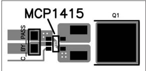
FIGURE 4-3: Recommended PCB Layout (TOP).
