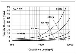
FIGURE 2-14: Supply Current vs. Capacitive Load.
