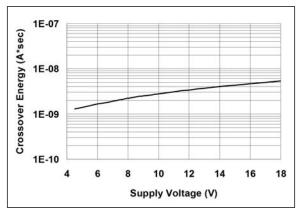
FIGURE 2-21: Crossover Energy vs. Supply Voltage.
