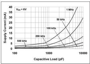
FIGURE 2-15: Supply Current vs. Capacitive Load.
