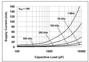
FIGURE 2-13: Supply Current vs. Capacitive Load.
