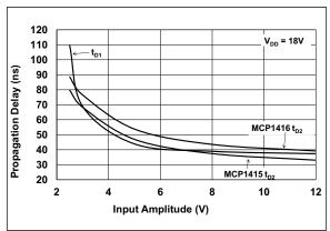
**FIGURE 2-6:** Propagation Delay Time vs. Input Amplitude.
