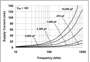
FIGURE 2-16: Supply Current vs. Frequency.
