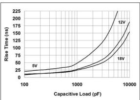
FIGURE 2-2: Rise Time vs. Capacitive Load.
