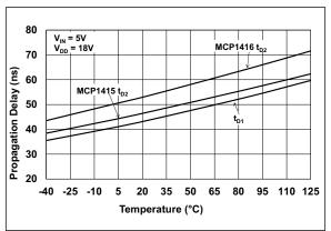
**FIGURE 2-8:** Propagation Delay Time vs. Temperature.
