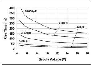
**FIGURE 2-1:** Rise Time vs. Supply Voltage.
