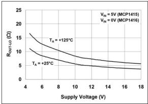
**FIGURE 2-20:** Output Resistance (Output Low) vs. Supply Voltage.
