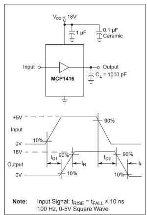
FIGURE 4-2: Non-Inverting Driver Timing Waveform.
