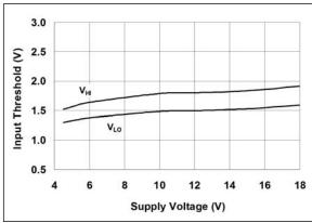
FIGURE 2-11: Input Threshold vs. Supply Voltage.
