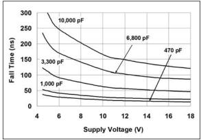
FIGURE 2-4: Fall Time vs. Supply Voltage.
