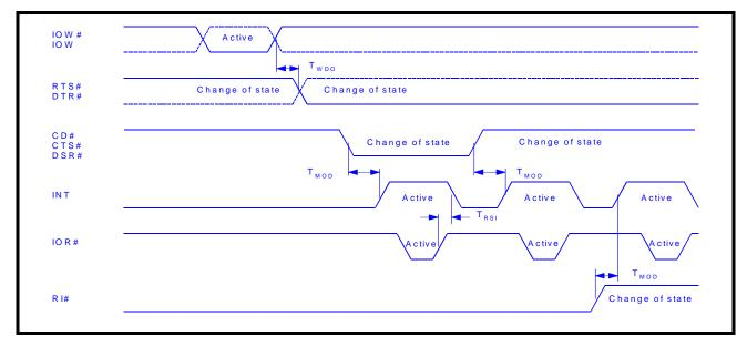
FIGURE 13. 16 MODE (INTEL) DATA BUS READ TIMING FOR CHANNELS A-D
